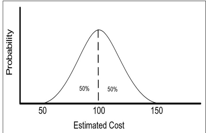
Figure 4—Variation of an estimate line item with normal probability distribution
