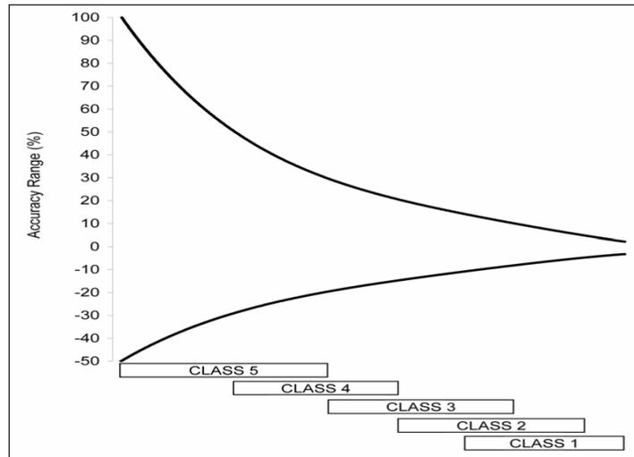
Figure 3—Estimate Accuracy Improves as the Level of Project Definition Improves
