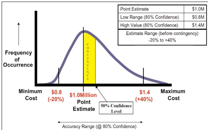
Figure 1—Estimate Accuracy Range around the Point Estimate
